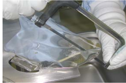
Fig. 6. Polished aluminum collector (it appears a hazy light blue because it reflects the blue cleanroom smock) secured to custom plate being hand- sawed.
