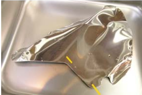
Fig. 3. Post-impact condition of polished aluminum collector. The yellow marks correlate with those on Fig. 5.
